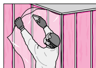
Applying air/vapour barrier
