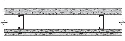
Partition Thickness: 4-1/8" (105 mm), Weight per Sq. Ft: 10 (49 kg/m<sup>2</sup>)
