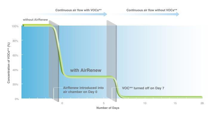
ISO 16000-23: Indoor air — Performance test for evaluating the reduction of formaldehyde concentrations by sorptive building materials. Third-party witnessed tests conducted at CertainTeed Research Center in Blue Bell, PA.
