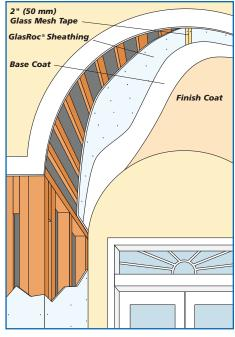
◀ Refer to finish system manufacturer for glass mesh reinforcement requirements.
